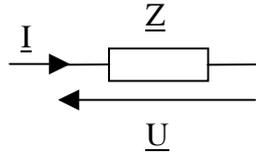
$$\underline{Z} = \frac{\underline{U}}{\underline{I}} = \frac{(U; \varphi_u)}{(I; \varphi_i)} = \left( \frac{U}{I}; \varphi_u - \varphi_i \right)$$
