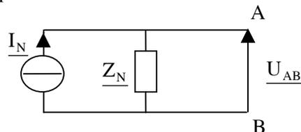
$$\underline{I}_N = (\underline{I}_{AB})_{\text{court-circuit}}$$
