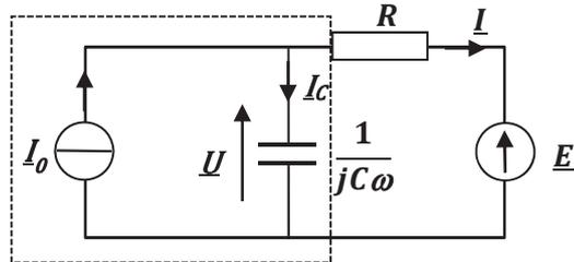
$$\underline{I}_0 = I_0 \exp\left(-j\frac{\pi}{2}\right) = -j I_0 \quad \text{et} \quad \underline{E} = E_0$$
